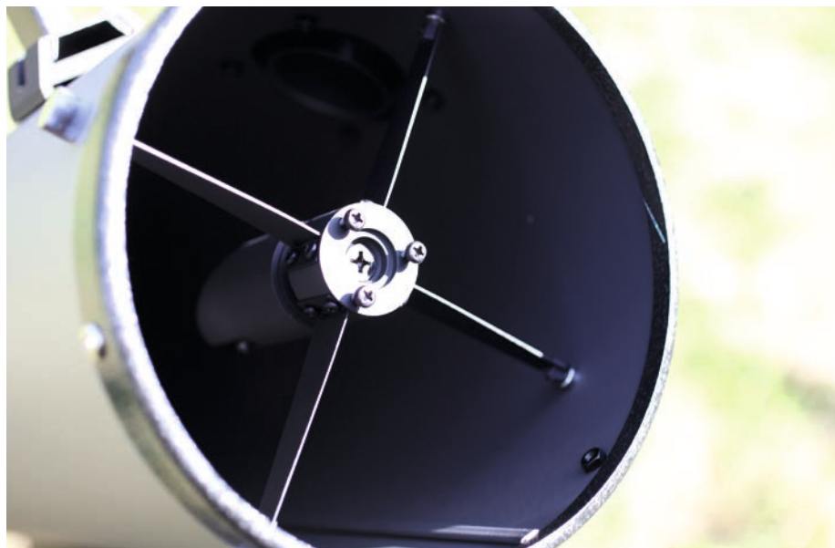
▲ The secondary and collimation adjustment is supported by the classical four vanes.
