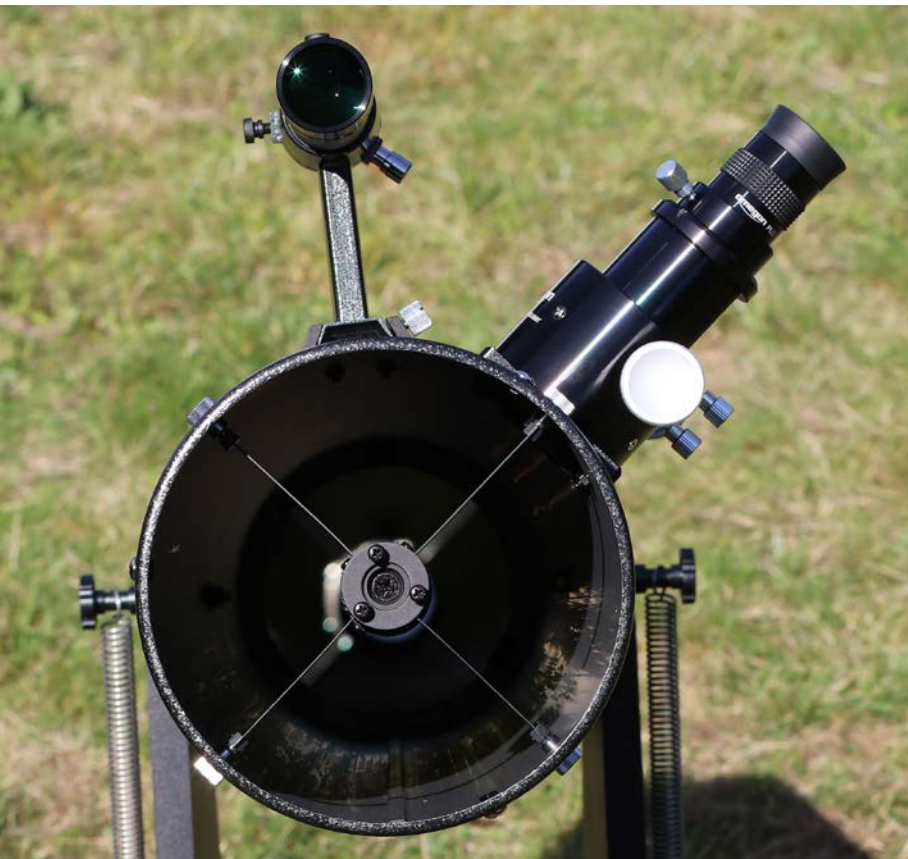
▲ Down the tube of the 152mm Newtonian.
