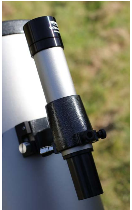
▲ The 6 × 30mm finder. Alignment is via twin screws against an opposing spring.
