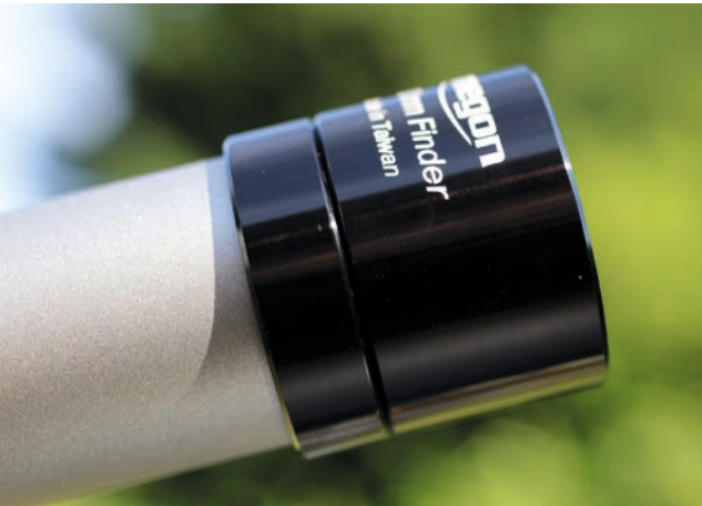
▲ The finder focuses by means of moving the objective lens on its threaded attachment.
